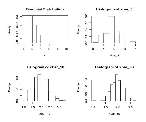
Explanation: X is a random variable with Binomial distribution (i.e., X~binom(10, 0.2)). The upper left panel shows what its (theoretical) probability distribution looks like; it is asymmetric and skewed right. We choose repeated samples (i.e., 500 samples) with sample size 3, 10 and 30, respectively. The rest of three histograms show the distribution of the sample average (when n = 3, 10 and 30), what do you observe?
